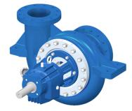
Centerline mounted, single-stage, overhung **Capacity:** 11,000 gpm / 2,500 m<sup>3</sup>/h **Head:** 1,250 ft / 380 m **Pressure:** 3,045 psig / 210 bar **Temp Range:** -150°F (-100° C) to 850° F (450° C) **Speed:** 3,600 rpm
