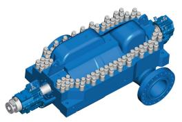
Axially split, volute or diffuser, single or double suction, between bearings **Capacity:** 8,800 gpm / 2,000 m<sup>3</sup>/h **Head:** 8,200 ft / 2,500 m **Pressure:** 2,175 psig / 150 bar **Temp Range:** -22°F (-30° C) to 390° F (200° C) **Speed:** 3,600 rpm
