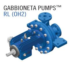
Centerline mounted, single-stage, low flow Barske type Capacity: 65 gpm / 15 m<sup>3</sup>/h Head: 656 ft / 200 m Pressure: 580 psig / 40 bar Temp Range: -150°F (-100° C) to 850° F (450° C) Speed: 3,600 rpm
