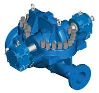
Axially split, single and two stage, double suction, between bearings Capacity: 53,000 gpm / 12,000 m<sup>3</sup>/h Head: 2,500 ft / 760 m Pressure: 870 psig / 60 bar Temp Range: -22° F (-30° C) to 390° F (200° C) Speed: 3,600 rpm
