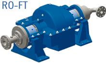
Pitot tube, between bearings Capacity: 450 gpm / 102 m<sup>3</sup>/h Head: 4,920 ft / 1,500 m Pressure: 2,175 psig / 150 bar Temp Range: 250° F (120° C) Speed: 6,000 rpm
