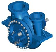
Radially split, single stage, double suction, between bearings Capacity: 53,000 gpm / 12,000 m<sup>3</sup>/h Head: 1,250 ft / 380 m Pressure: 1,450 psig / 100 bar Temp Range: -22°F (-30° C) to 850° F (455° C) Speed: 3,600 rpm
