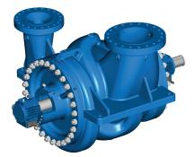
Radially split, single-stage, double suction, between bearings Capacity: 8,800 gpm / 2,000 m<sup>3</sup>/h Head: 2,500 ft / 760 m Pressure: 2,175 psig / 150 bar Temp Range: -22°F (-30° C) to 850° F (455° C) Speed: 3,600 rpm
