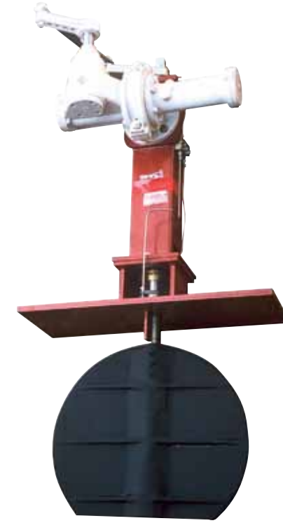
650mm valve for slotting into pipeworks. Lower segment of disc removed to clear tar deposits in line. Complete with Askania actuator used in a steel works.
