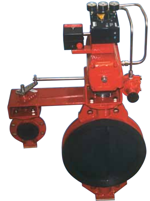
300mm and 50mm control valves with Mecair actuator mechanically linked for use on parallel lines at UK refinery.
