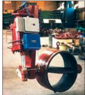
A 600mm butt weld design reheat steam balancing valve with cylinder and Babcock positioner and transmitter. Installed at Castle Peak Power Station, Hong Kong.
