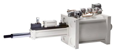
Tandem linear pneumatic actuators include all the features of our linear pneumatic actuators with the addition of a hydraulic cylinder to facilitate precise and repeatable speed control.
