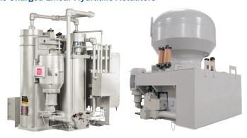
Gas charged linear hydraulic actuators are self-contained hydraulic actuators with integral nitrogen storage to provide a fast failsafe stroke. They are typically used for MSIV and MFIV applications.
