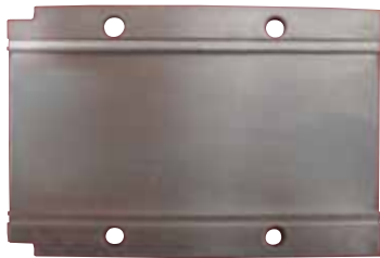
Blank disc simulates single stage trim
