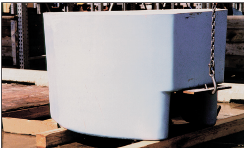
Step 7: After concrete has cured, use hoist plate* / fastout device** and suitable rigging*** to turn basin right-side up
