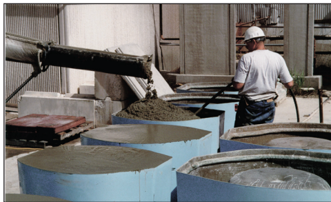
Step 5: Multiple shells may be filled simultaneously
